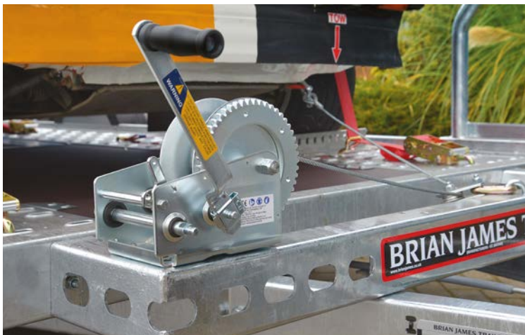
○ Manual winch + 3 point adjustable pull positions.
